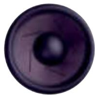
**Midrange** The twin midrange drive units that supply the bulk of Zeppelin's amazing sound rely on glass fibre cones, optimized using laser interferometry. Strategically placed resin-filled slots in the cones dramatically reduce the unwanted effects of standing waves, leaving music sounding cleaner, clearer and true to life.
