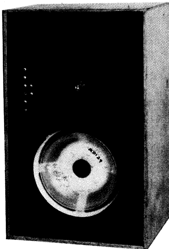
Fig. 1 — Prototype small monitoring loudspeaker type LS 5/9 with front grille removed.
